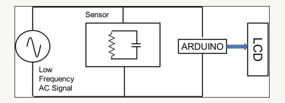
In the figure, the sensor behaves like a resistor which requires a low frequency AC input signal. The function of timer circuit is to produce a low frequency to support the cell inside the biosensor. After the detection, the impedance data will be taken based on day 1, day 2 and so on. The impedance data is proposed to be measured using the Arduino system and the value is then displayed using an LCD
