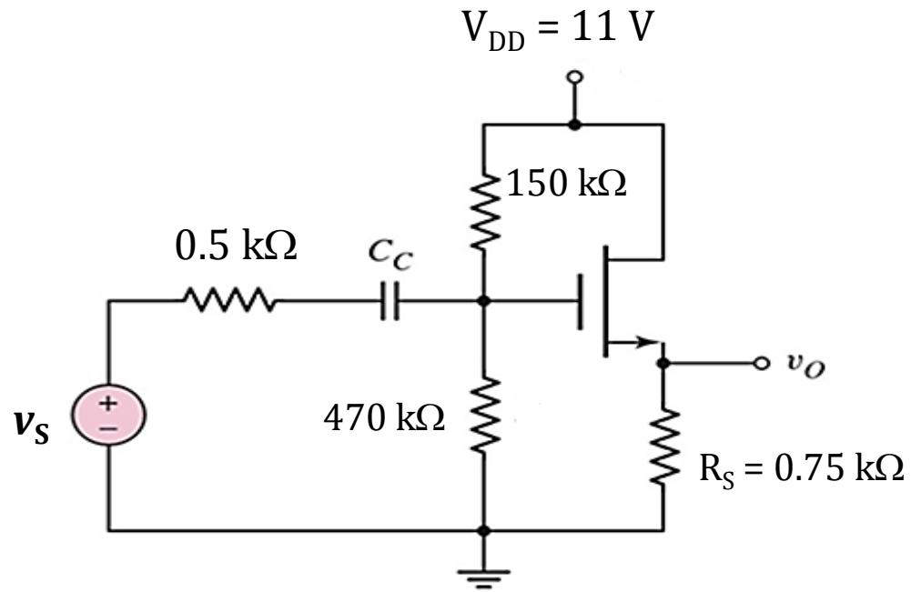
$$V_{TN} = 0.92 \text{ V}, K_n = 4 \text{ mA/V}^2, \lambda = 0.01 \text{ V}^{-1}$$
