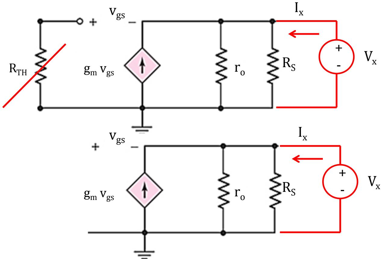
$v_{gs}$  in terms of  $V_x$  where  $v_{gs} = -V_x$
