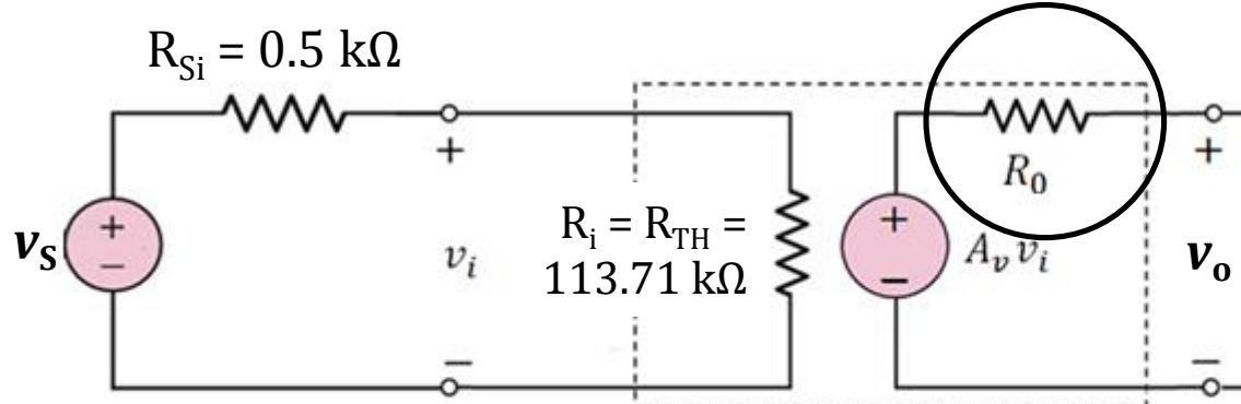
Equivalent circuit of a voltage amplifier
