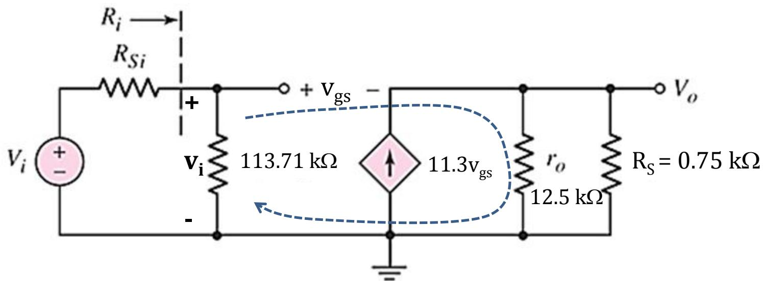
1. The output resistance:  $R_{eq} = r_o \parallel R_s = 0.70755 \text{ k}\Omega$
