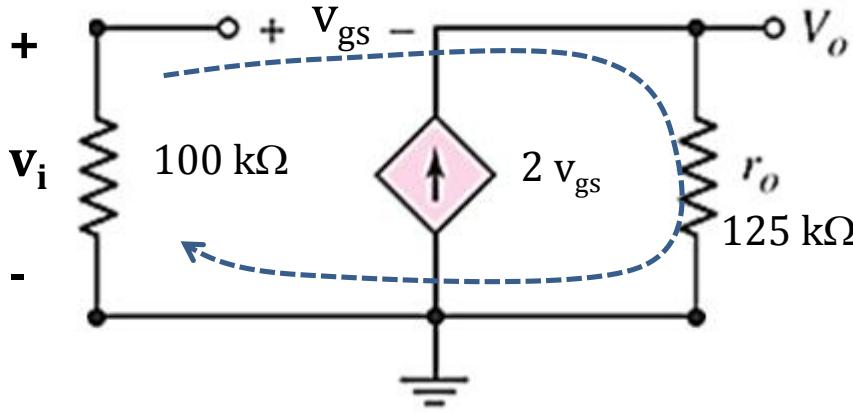
1. The output resistance:  $R_{eq} = r_o = 125 \text{ k}\Omega$
