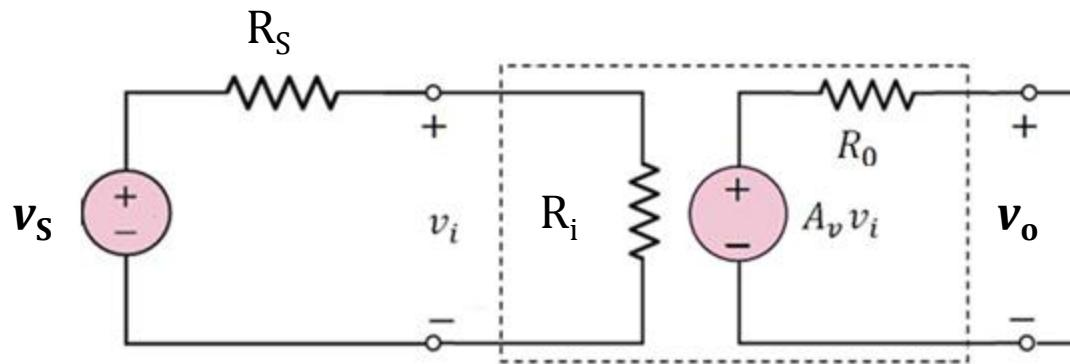
Equivalent circuit of a voltage amplifier
