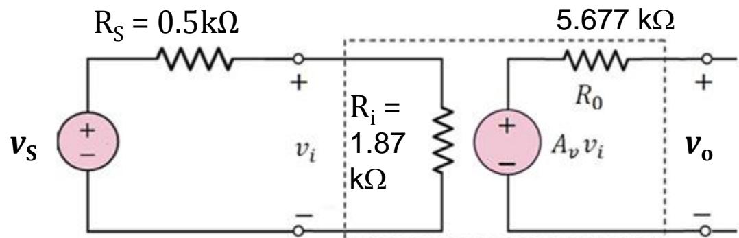
Equivalent circuit of a voltage amplifier
