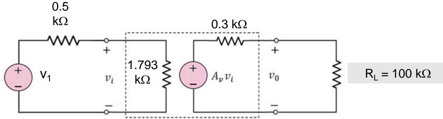
To find new voltage gain,  $v_o/v_1$  now with signal voltage,  $v_1$  and  $R_L$
