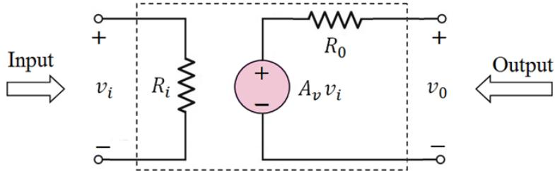
Equivalent circuit of a voltage amplifier
