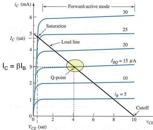
Q-point is the intersection of the load line with the  $i_C vs v_{CE}$  curve, corresponding to the appropriate base current
