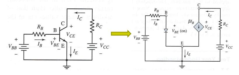
Assume that the B-E junction is forward biased, so the voltage drop across that junction is the cut-in or turn-on voltage  $V_{BE}$  (on).
