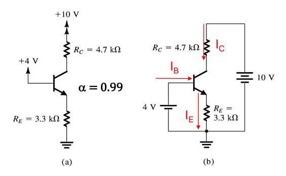
KVL at BE loop:  $0.7 + I_E R_E - 4 = 0$  $I_E = 3.3 / 3.3 = 1 \text{ mA}$
